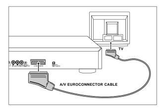
Connection to a TV with an A/V Euroconnector socket.
